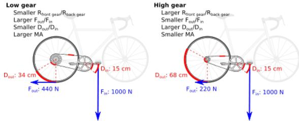
Mechanical advantage in different gears of a bicycle. Note that even in low gear the MA of a bicycle is less than 1 because what we want is movement, not force on the wheel.
